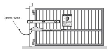
The operator can be mounted on top of the gate frame.
