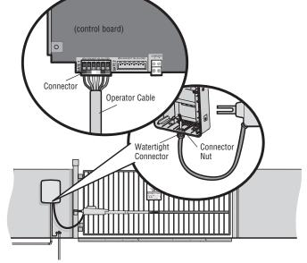
If installing one operator, proceed to page 20. If installing two operators, go to the following page.
