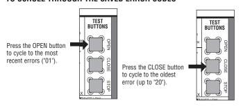
The operator will only keep track of up to 20 errors, then will start saving over the oldest errors as new errors occur.
